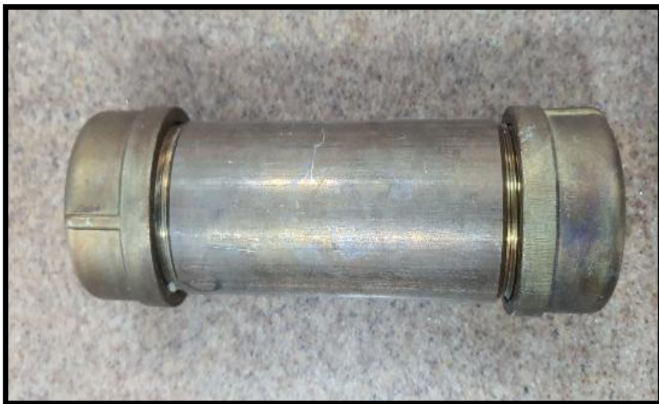
Figure (25): An iron capsule for charcoal leaf powder, cloves, marmaki and al-jowaifa sweetened at a temperature 450\text{ C}^{\circ}
